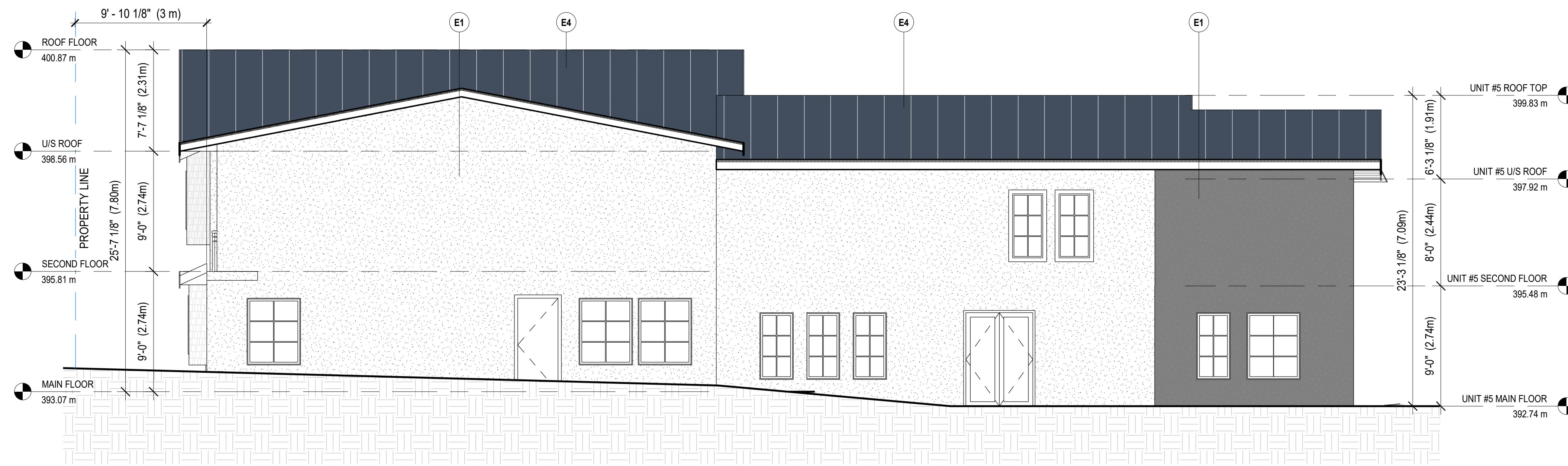
3 UNIT #5, #6 & #7 NORTH ELEVATION A 3.02 3/16" = 1'-0"
